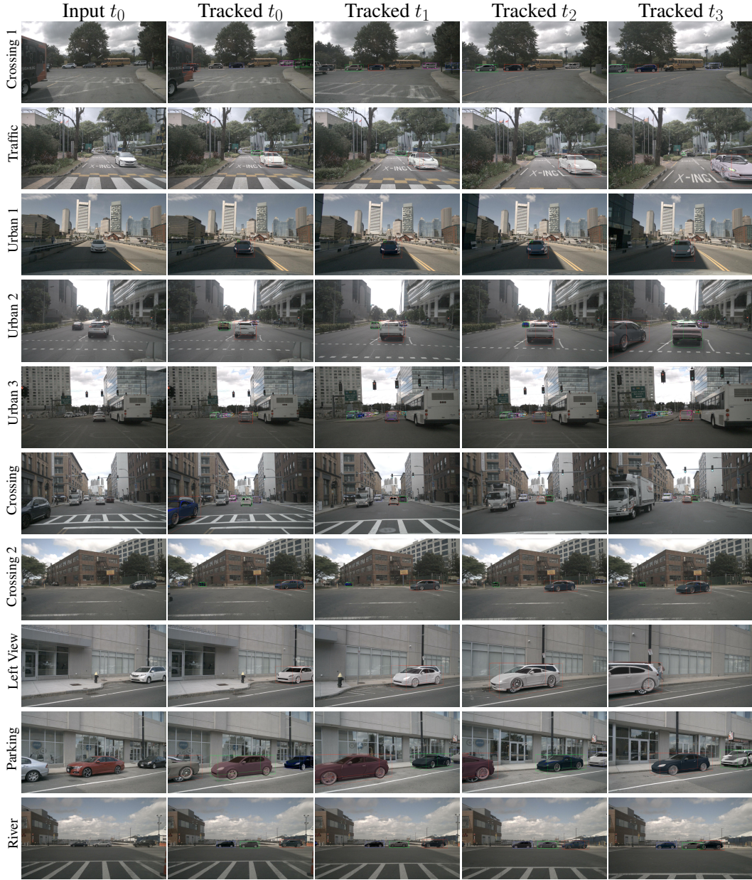
Supplementary Figure 1: Additional visualizations on nuScenes 1 . From left to right, we show (i) observed images from diverse scenes at timestep k = 0 ; (ii) an overlay of the optimized generated object and its 3D bounding boxes at timestep k = 0, 1, 2 and 3. The color of the bounding boxes for each object corresponds to the predicted tracklet ID. We see that our method can accurately reconstruct objects in diverse scenarios.
