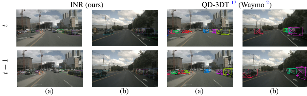
Supplementary Figure 7: Qualitative Comparison on Generalization. We compare 3D bounding box outputs from QD-3DT 17 end-to-end trained on Waymo Open Dataset 2 and our inverse neural rendering-based tracker (INR) overlaid on the respective input videos from nuScenes 1 . The same color in consecutive frames denotes the same tracklet. As we see in scene (a) on the left side QD-3DT has ID switches especially in the far range and on the sides of a frame implying dataset-specific performance caps, e.g. the training dataset has been tracking annotated in a rather short range. Another finding is exemplified in scene (b) on the right side where the tracker does not generalize well and is losing a tracklet.
