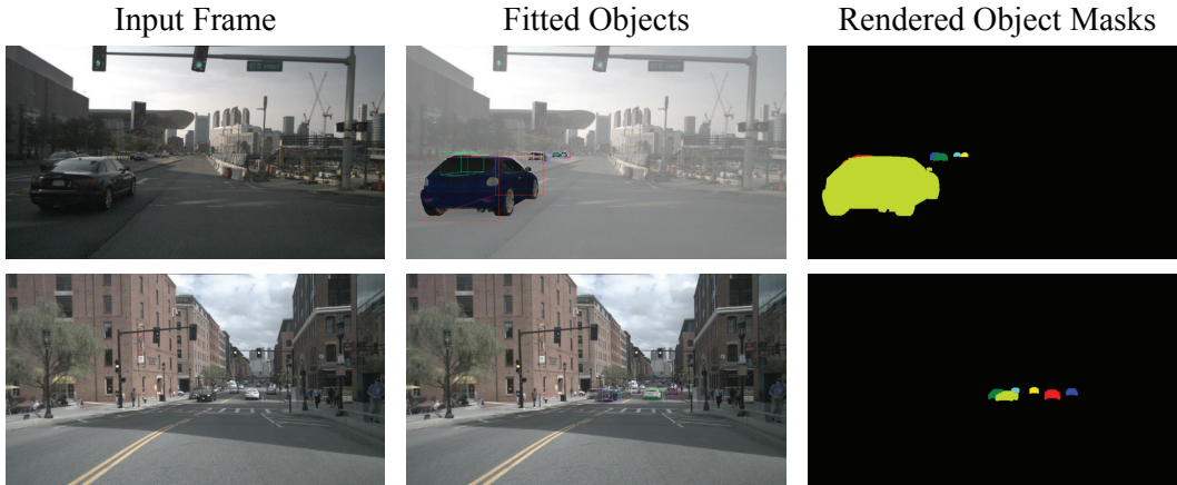
Supplementary Figure 9: Rendered Instance Segmentation. Coarse instance segmentation can be directly obtained from the rendering pipeline for free. For each fitted object, we additionally render a depth-ordered alpha mask. This can be used to assign a per-pixel instance segmentation masks as shown on the right.
