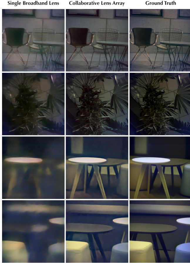
Fig. 9. Comparison between a single broadband-optimized lens and the proposed collaborative array under challenging illumination spectra. Although a single metalens can be continuously optimized for broadband illumination within our framework (left), a single lens struggles to focus the entire visible spectrum. In contrast, our method employs multiple collaboratively optimized lenses to overcome these limitations. We confirm this here qualitatively with reconstructions under challenging illumination scenarios—such as heavily tilted spectra or discrete illumination [Li et al. 2021]—demonstrating that our collaborative array design consistently outperforms the single broadband lens across a variety of illumination conditions, see text.
