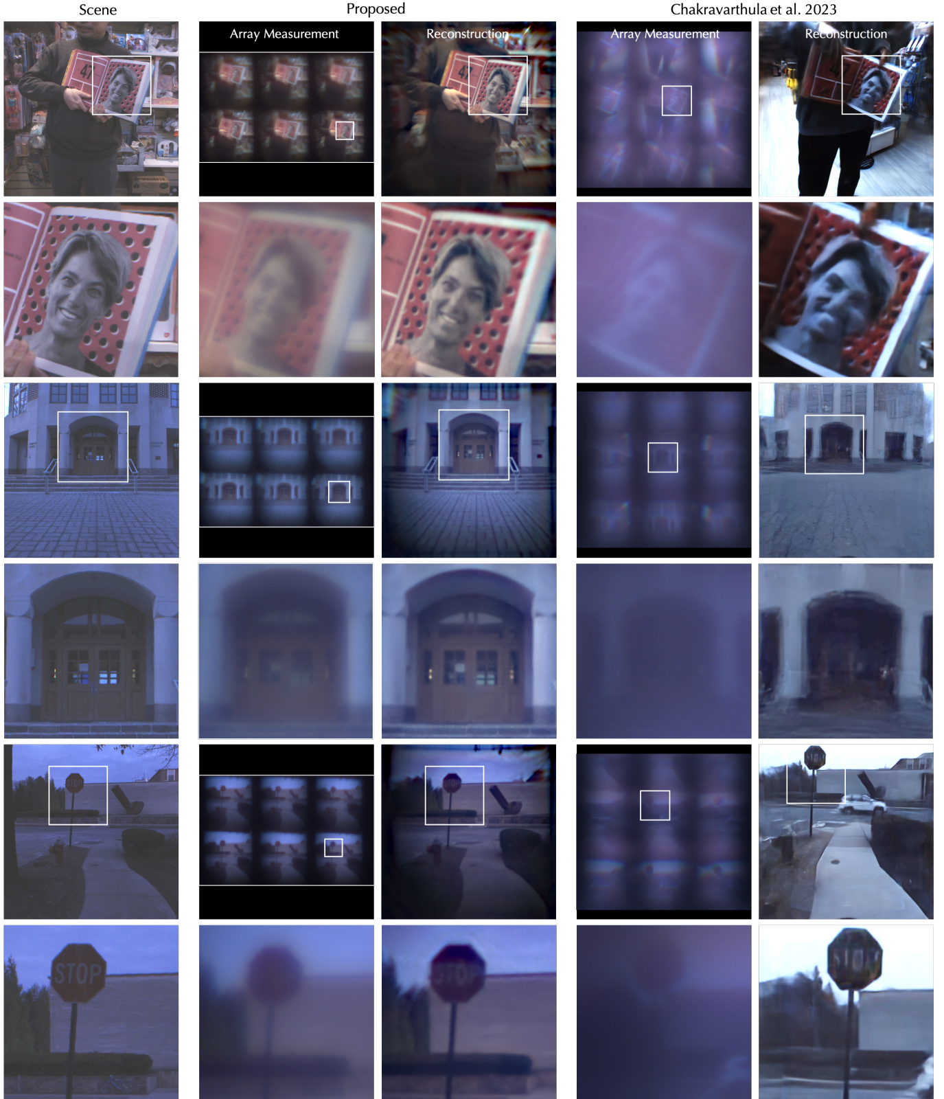
Fig. 12. Experimental comparison to [Chakravarthula et al. 2023]. For similar scenes and illumination conditions, the proposed collaborative metalens array provides more accurate measurements and image reconstructions than [Chakravarthula et al. 2023]. The image zoom-ins show the proposed collaborative metalens array can capture a more broadband focused raw measurement, and a more plausible reconstruction of the scene, revealing details such as the portrait, building door windows, and a stop sign.
