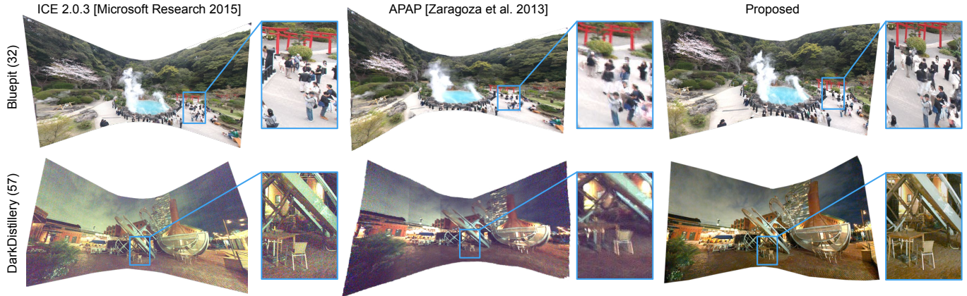
Fig. 8. Image Stitching Comparisons. Visualizing rectilinear projections of the stitched panoramas, we see that APAP [Zaragoza et al. 2013] averages multiple frames in DarkDistillery to reduce noise, while ICE [Microsoft Research 2015] segments and freezes the motion of pedestrians in Bluepit . Our proposed approach aims to do both, averaging multiple rays to reduce noise when possible while also preserving content in areas with local scene motion.
