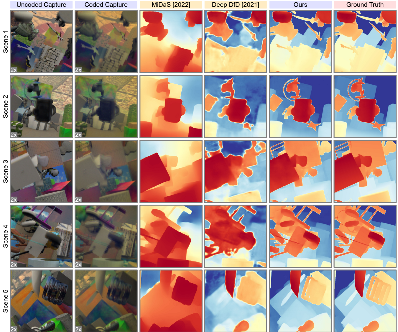
Fig. 10. Additional Synthetic results of Monocular Depth Imaging. We assess our approach for monocular depth estimation in simulation by comparing our method to the monocular depth estimation method MiDaS [Ranftl et al. 2022], and DOE-based depth from defocus method Deep DfD [Ikoma et al. 2021]. While MiDaS estimates a qualitatively plausible depth map, their estimation remains relative and misrepresent the spatial relationship of non-adjacent objects . Deep DfD, capable of recovering depth scale, faces challenges in resolving fine details. Our method, leveraging both the sharp details from the in-focus uncoded capture and the depth cues from the coded captures, is able to accurately capture both the scale and details in the scene.
