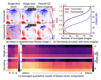
Figure 5. Noise in Stokes images and intensity denoising. (a) Stokes vector  $s_1$  reconstructed from a single-shot, single-shot with a learned intensity denoiser [66], and burst imaging (Pseudo GT) averaged over 100 shots. (b) Reconstruction accuracy of a Stokes image with varying number of averaged images. (c) Reconstruction accuracy of Stokes elements with and without intensity denoising.
