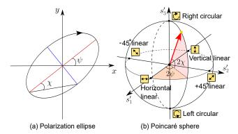
Figure 1. Two representative polarization visualizations. (a) Polarization ellipse depicts the electric-field oscillation projected onto a plane tangent to the light propagation. (b) Poincaré sphere visualizes the polarization state of light on the normalized Stokesvector axes  $s'_1$ ,  $s'_2$ ,  $s'_3$ .
