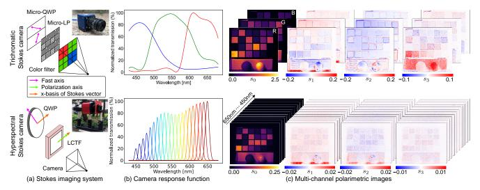
Figure 3. **Acquisition of spectro-polarimetric images.** We capture spectro-polarimetric images using (a) trichromatic and hyperspectral Stokes cameras [34, 57]. (b) Camera response functions. (c) Reconstructed raw Stokes images per each spectral channel.
