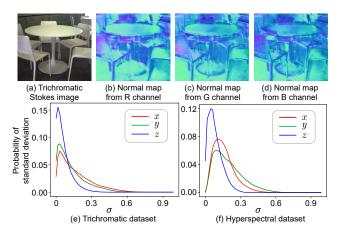
Figure 9. **Spectral dependency of conventional SFP method.** (a) Trichromatic Stokes image and estimated surface normals [41] for each red, green, and blue spectral channels shown in (b), (c), and (d). Graphs (e) and (f) show the probability distributions of standard deviation of normal component x, y, and z along the spectral channels for both datasets.
