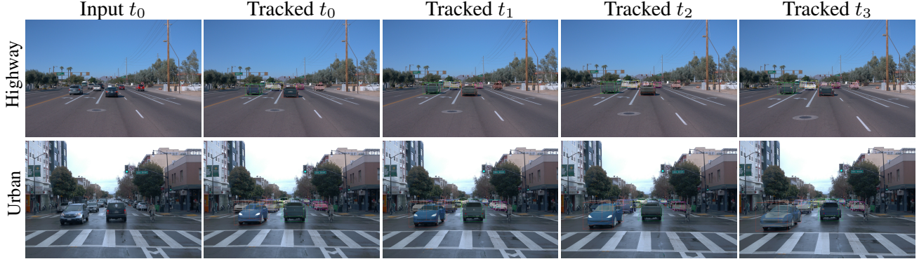
Figure 3. Without changing the model or training on the dataset, our proposed method can generalize well to the Waymo Open Driving Dataset [67]. Similar to Fig 2, from left to right, we show (i) observed images from diverse scenes from the dataset at timestep k = 0 ; (ii) an overlay of the closest generated object and predicted 3D bounding boxes at timestep k = 0, 1, 2 and 3. The color of the bounding boxes for each object corresponds to the predicted tracklet ID. Our method does not lose any tracks even on a different unseen dataset in diverse scenes, validating that the approach generalizes.
