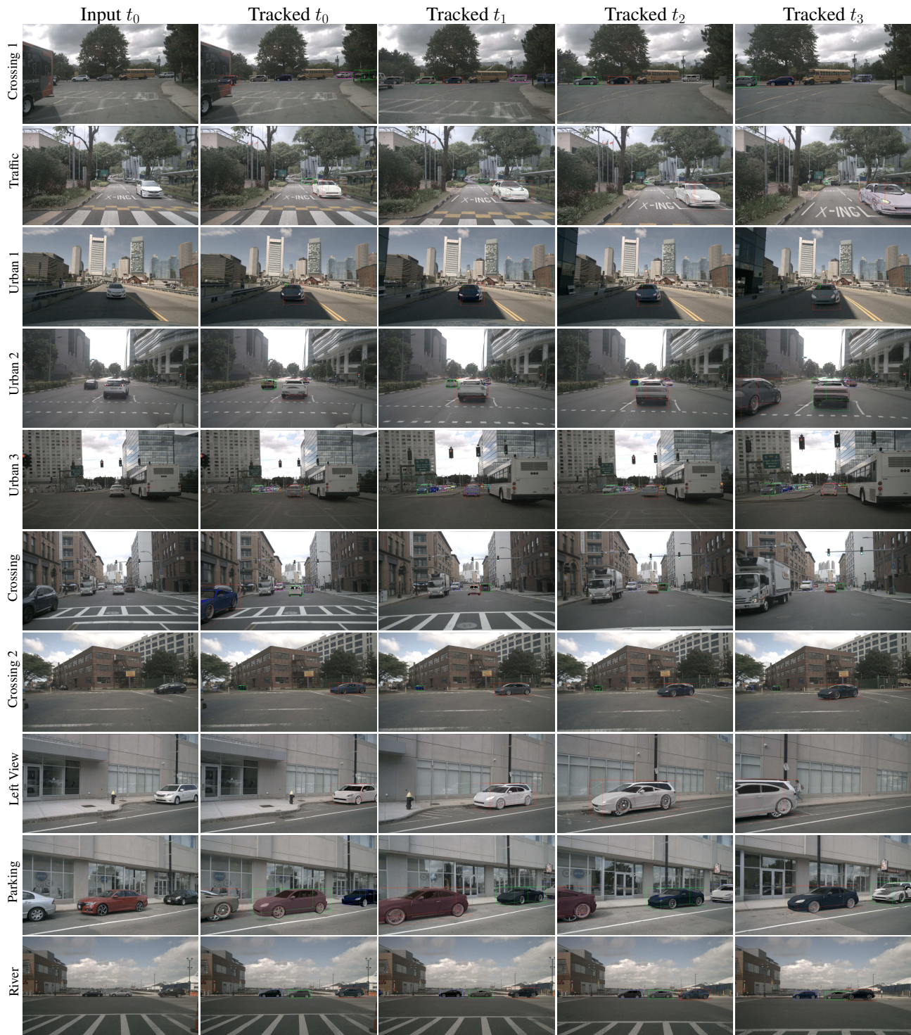
Figure 4. Additional visualizations on nuScenes [1]. From left to right, we show (i) observed images from diverse scenes at timestep k = 0 ; (ii) an overlay of the optimized generated object and its 3D bounding boxes at timestep k = 0, 1, 2 and 3. The color of the bounding boxes for each object corresponds to the predicted tracklet ID. We see that our method can accurately reconstruct objects in diverse scenarios.
