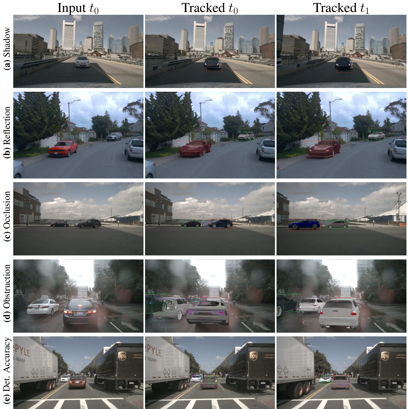
Figure 2. Examples of failure cases, such as lighting (shadows and reflections) or occluded objects, where the reconstructed object differs significantly from the observed object. These visualizations allow us to understand exactly why our model fails at reconstructing and tracking objects. This also allows us to identify ways the representation model and perception pipeline can be improved to incorporate effects that cause the method to fail.
