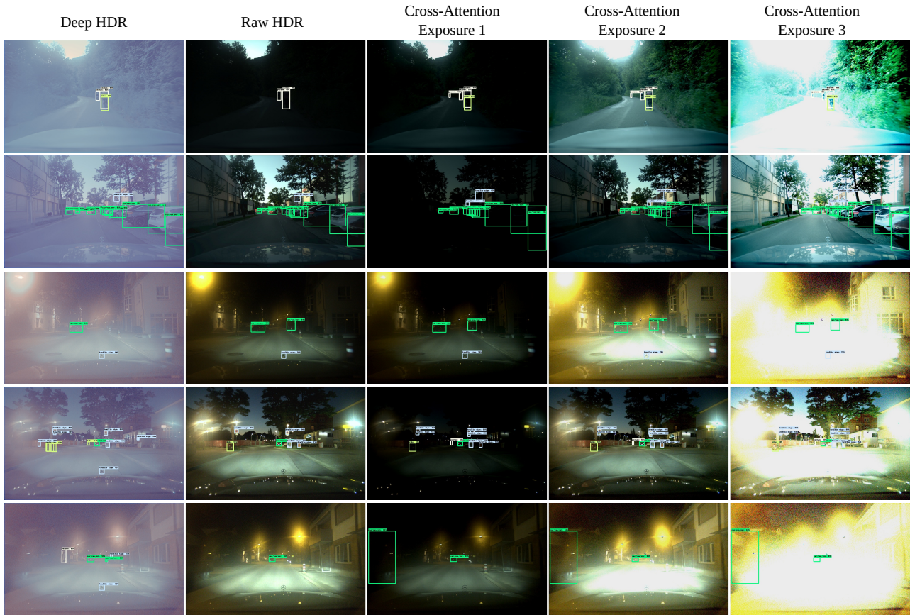
Figure 3. Qualitative comparison of the proposed Local Cross-Attention Fusion with the baseline methods Raw HDR and Deep HDR [6] on challenging scenes. Our neural fusion module recover features from separate exposure streams to support vision the downstream vision task.
