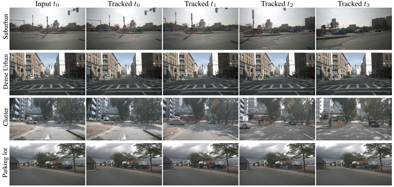
Figure 2. Tracking via Inverse Neural Rendering on nuScenes [7]. From left to right, we show (i) observed images from diverse scenes at timestep k = 0 ; (ii) an overlay of the optimized generated object and its 3D bounding boxes at timestep k = 0, 1, 2 and 3. The color of the bounding boxes for each object corresponds to the predicted tracklet ID. We see that even in such diverse scenarios, our method does not lose any tracks and performs robustly across all scenarios, although the dataset is unseen.
