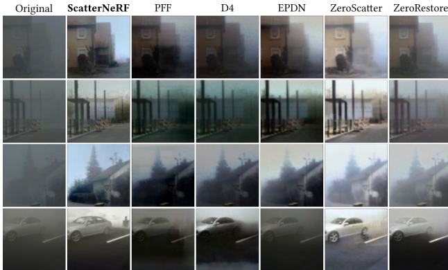
Figure 5: Qualitative comparison of dehazed images on real-world automotive measurements. The proposed ScatterNeRF enables enhanced contrast and visibility compared to state-of-the-art descattering methods.
