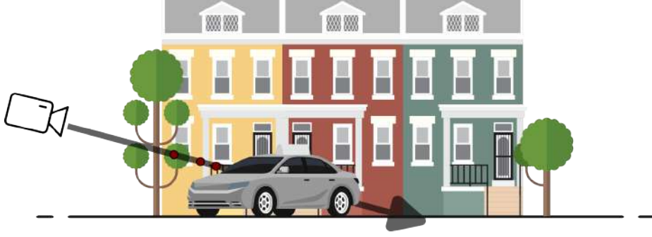
Figure 1: Schematic visualization of the neural rendering approach. For a camera position, the scene is integrated along one camera ray \mathbf{r} (gray) at the sampled red positions. Hereby, the interactions along the ray model the scene’s appearance in the image.
