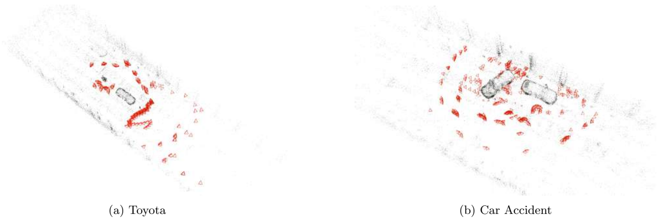
Figure 11: Distribution of camera poses in the controlled environment dataset. The position and heading of the camera is visualized with red frustums. For visualization purposes we show the camera poses in context of the sparse point cloud estimated by hloc.
