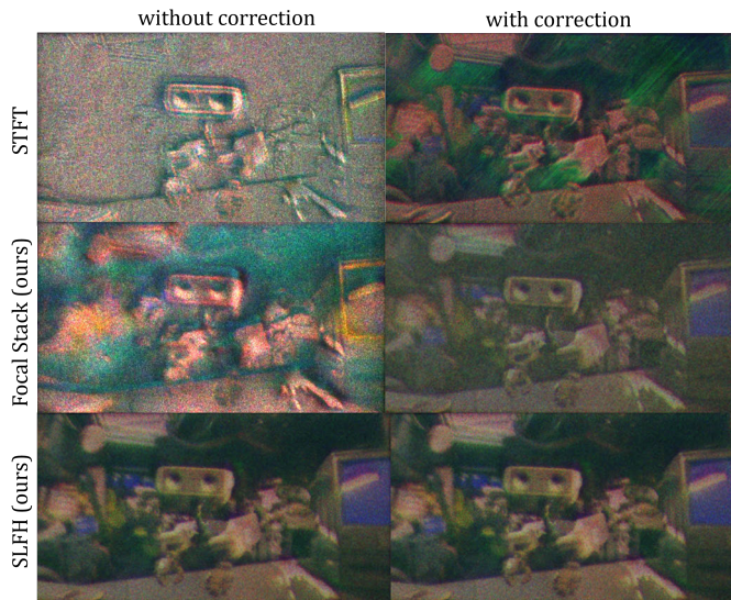
Fig. 10: Artefacts in competing methods with and without no-care-areas at the edge of the eye-box (Experiment). Plain STFT/Focal-Stack cannot produce holograms at close propagation distances (left). Only by introducing a band-pass filter during propagation (right), we can compute holograms for those. Even with correction, at the edge of the eye-box, STFT and FS strong artifacts streak artifacts or noisy images, respectively.
