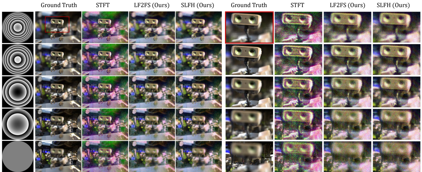
Fig. 6: Experiment: Focal-stack evaluation: We show experimental results for SOTA algorithms evaluated with a wide open aperture and defocus varying from z \in [0mm, 13mm] . The STFT training method produces significant color artifacts, while our new SLFH method and our implementation of Focal Stack supervision (LF2FS) produce high quality results with similar performance.
