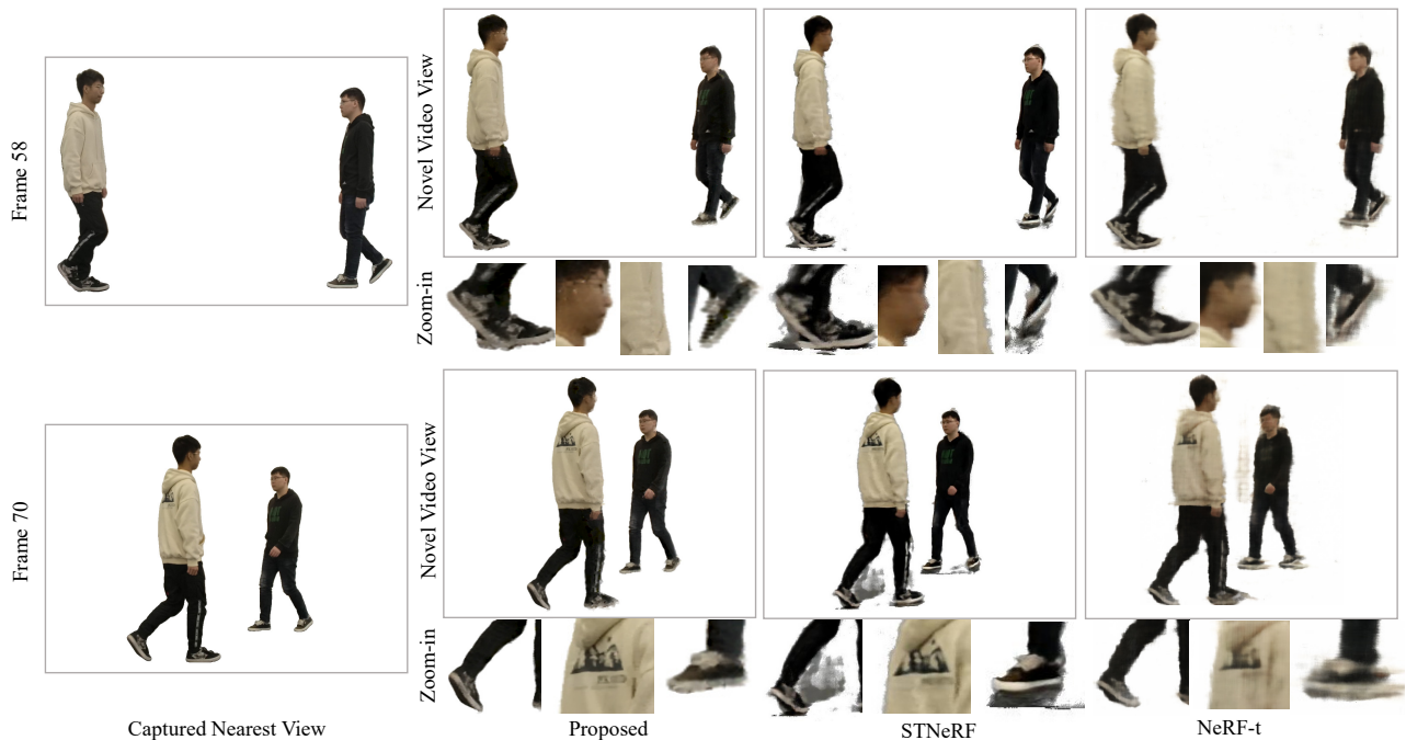
Figure 4: Novel Video View Synthesis. We synthesize novel views for video timestamps of the STNeRF [2021] dataset (Frame 58 and Frame 70). Compared to STNeRF [2021] and the NeRF-t model proposed in the same work, the differential point cloud radiance field approach produces substantially cleaner object boundaries, finer object detail and fewer reconstruction artifacts, especially in the presence of significant object motion, as illustrated in the insets.
