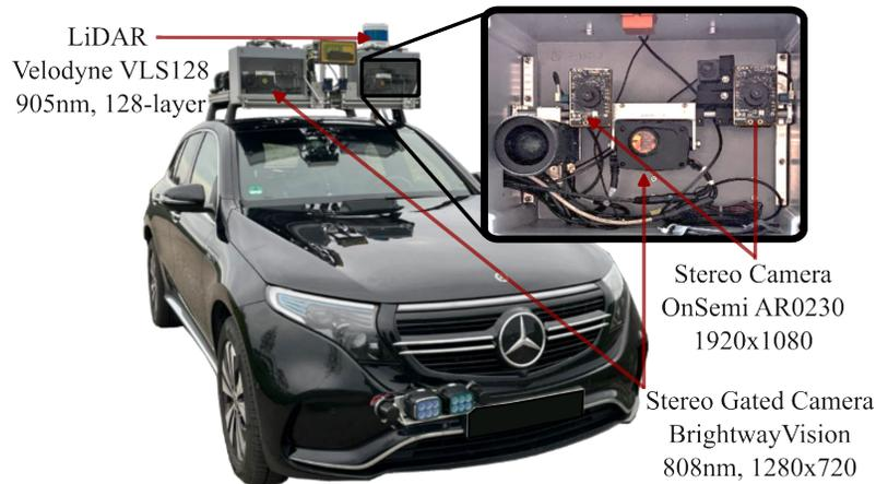
Figure 1. Experimental sensor setup of the prototype vehicle for data acquisition. The car is equipped with a stereo gated imaging system with a baseline of 0.76 m, consisting of two gated imagers and a flood-light flash source, a standard RGB automotive stereo camera and a scanning LiDAR Velodyne VLS128 as reference.
