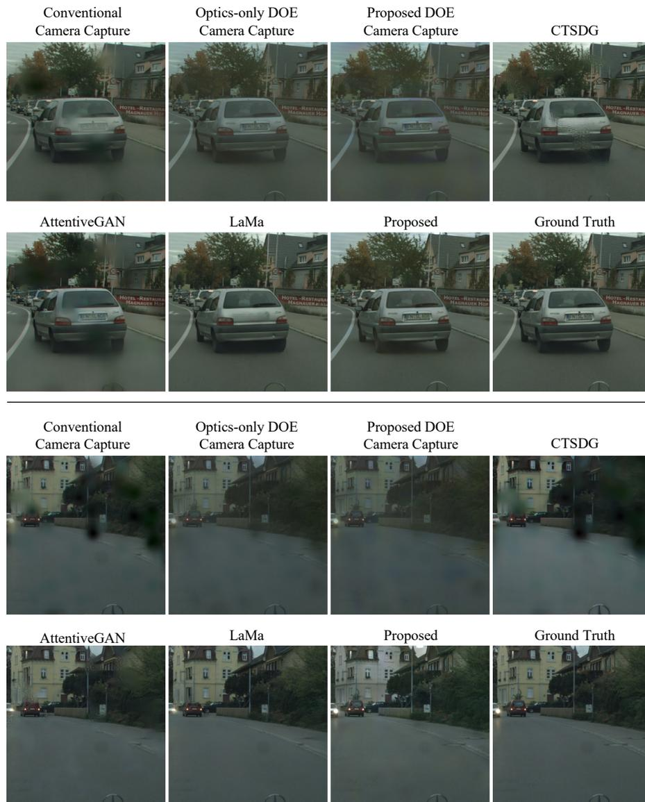
Fig. 6. **Additional rain-drop obstructions results.** Our DOE (optimized to operate with or without a subsequent neural network) allows us to see through occlusions. Feeding the captured image into our neural network results in an almost obstruction-free image. Existing inpainting methods (CTSDG and LaMa), as well as a designated raindrop removal AttentiveGAN method [Qian et al. 2018], often fail to reconstruct important visual details, e.g. license plates in both examples.
