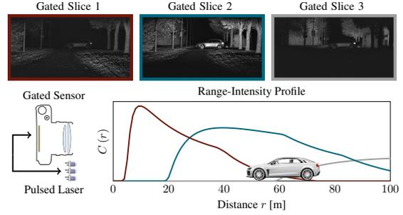
Figure 2: A gated system consists of a pulsed laser source and a gated imager that are time-synchronized. The range-intensity profile (RIP)  $C_i(r)$  describes the distance-dependent illumination for a slice  $i$ . A car at a certain distance appears with a different intensity in each slice according to the RIP.
