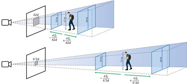
Figure 4: There is an infinite number of 3D cuboids that can project to a given bounding box  $P$ . However, the object location can be reasonably estimated using the object height, its projected height, and the vertical focal length.
