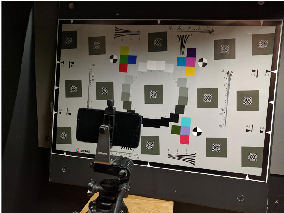
Fig. 4. Noise calibration setup.
