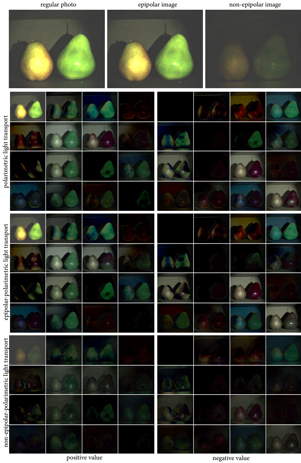
Fig. 15. Additional spatio-polarimetric decompositions. The top row shows a conventional photography and the corresponding epipolar/non-epipolar captures [O’Toole et al. 2012]. The second row shows the polarimetric reconstructions [Azzam 1978]. The bottom two rows show the epipolar- and non-epipolar-polarimetric reconstructions.
