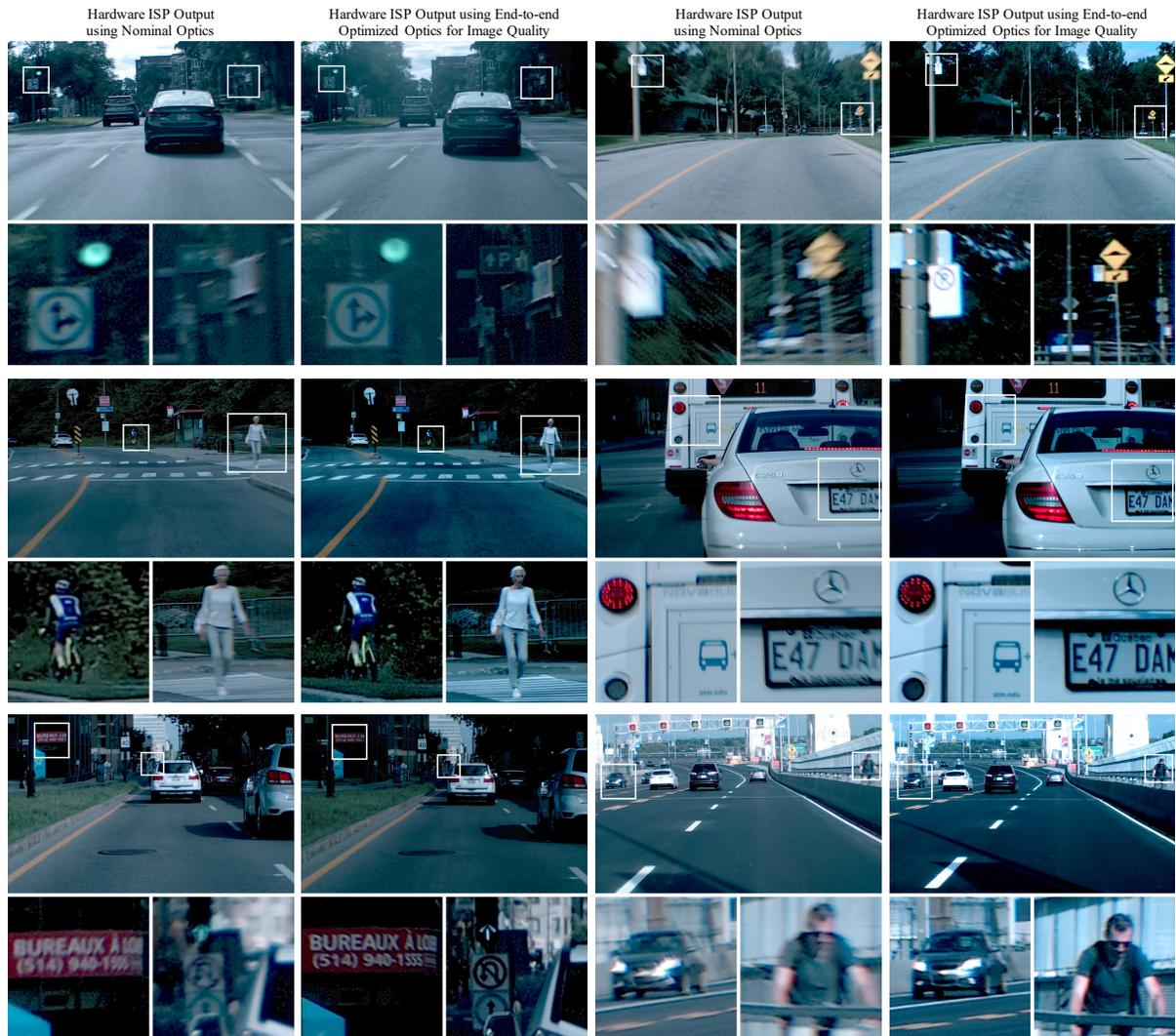
Fig. 22. Real-world prototype captures for image quality with Cooke triplet and hardware ISP. The image pipeline using the manufactured optimized optic produces sharper results in the periphery and similar quality results in the center.
