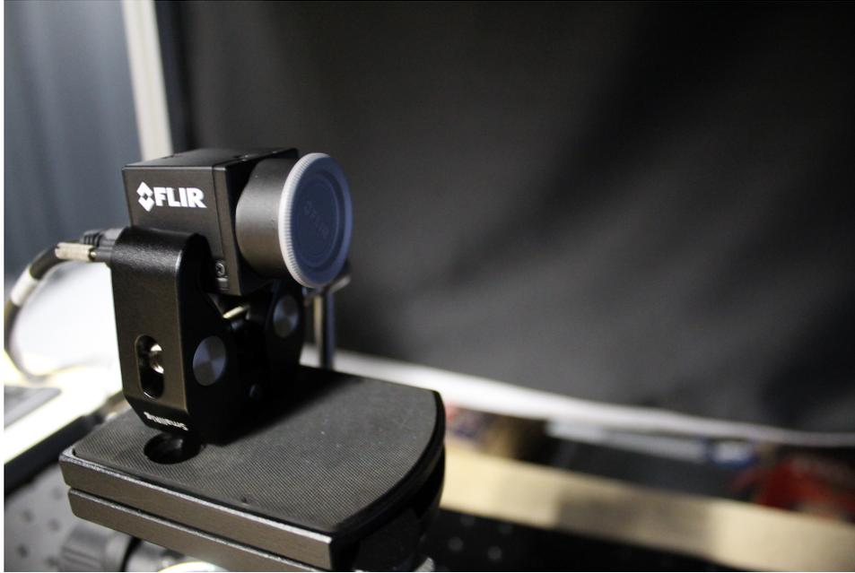
Fig. 3. Camera was covered with an opaque surface to take the dark frames.
