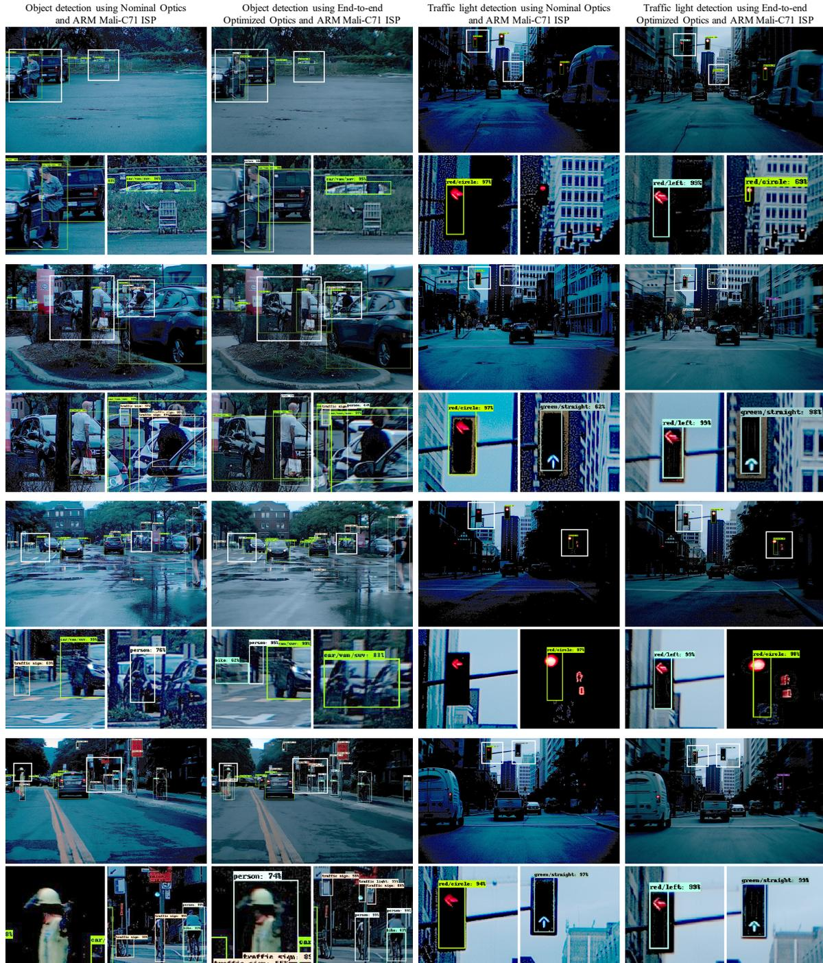
Fig. 23. Real-world prototype captures for automotive object and traffic light detection with Cooke triplet and hardware ISP. The optimized optics have greater light efficiency (smaller f-number) and more uniform blur across the field of view than the nominal optic, which leads to greater detection performance. Note that the traffic light detection captures were taken at dusk.
