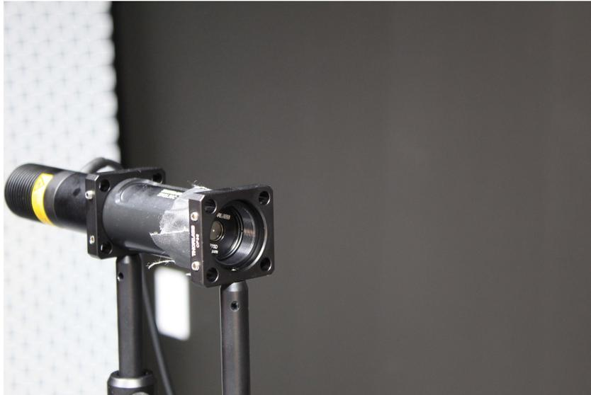
Fig. 32. Pin-hole light source setup.
