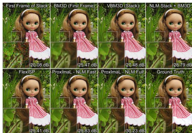
**Figure 9:** Comparison of image priors for burst denoising & demosaicking. For this simulation, a non-local means (NLM) prior outperforms the BM3D prior. The approximate NLM implemented in OpenCV is faster than, but not quite as good as, a full implementation.<sup>3</sup>
