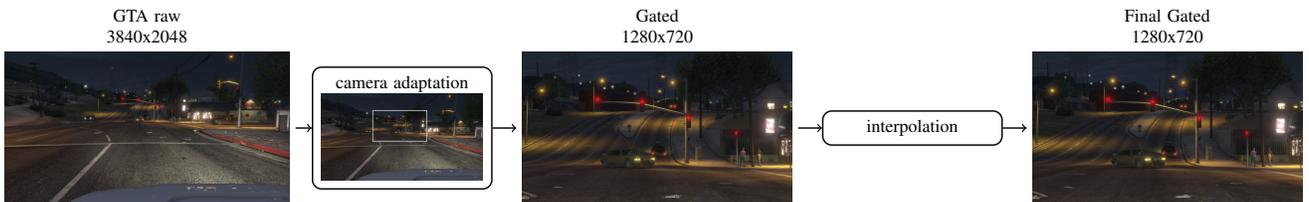
Figure 3: Steps for adapting the intrinsic calibration and resolution from the original GTA camera to the gated camera.
