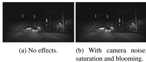
Figure 8: We include three important camera effects: noise, saturation and blooming. This figure shows the influence of these components.
