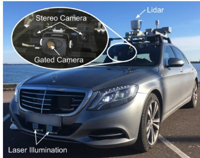
Figure 9: The sensor setup of our test vehicle for validation is shown. The car is equipped with a gated camera, consisting of a flood-light flash source, gated imager and a scanning lidar Velodyne HDL64-S3D as reference.
